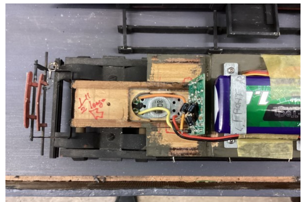
Horn sound card, speaker & servo switch were in roof arc cavity, now on frame near front bogie.
