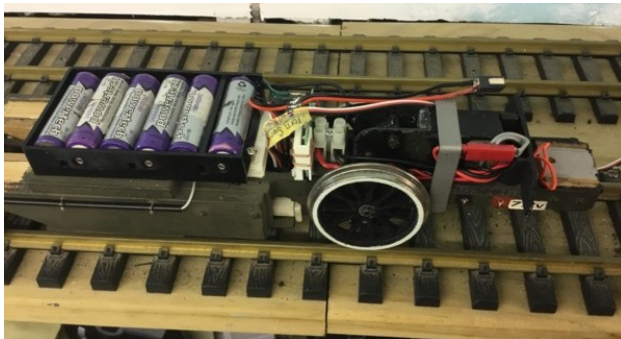
The 6 cells AA NiMH (7.2 volts) sat over the Rx. Update, in 2023 a 2S nano tech 1000mAh LiPo was used to replace the 6 AA NiMH cells in a tray.
